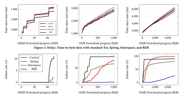
Figure 3: Failure rate: Percentage of attempted downloads that failed with standard Tor, REB, Spring, and Interspace
