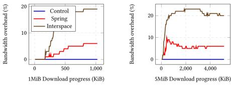
Figure 1: Bandwidth overhead: Median of receive bandwidth overhead with standard Tor, Spring, and Interspace
